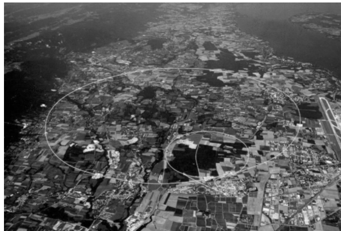
Figure 1. Aerial view of the CERN underground accelerator complex. The larger ring, 27 km long, will house the Large Hadron Collider. On the right, the runaway system of the Geneva International Airport and a portion of Lake Geneva give an idea of the scale.
